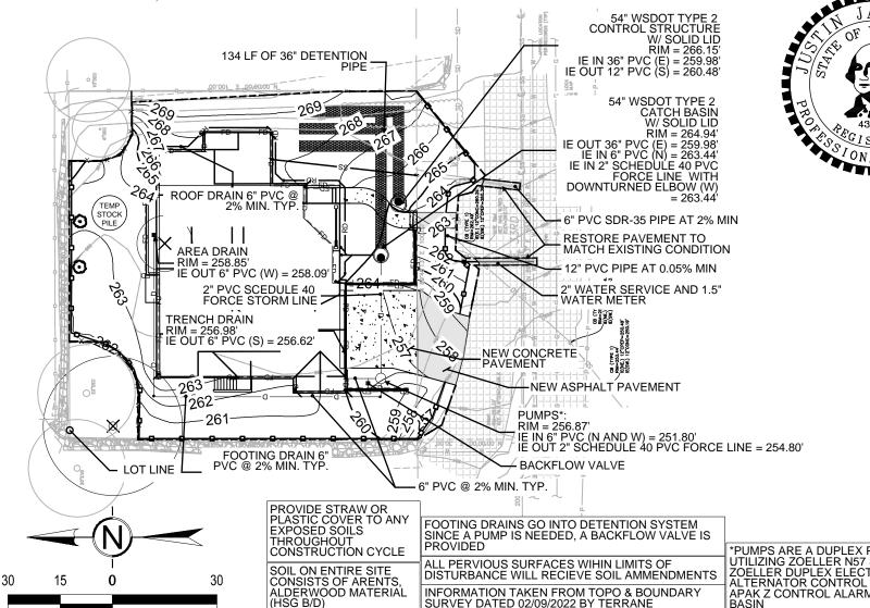
\*PUMPS ARE A DUPLEX PUMP SYSTEM UTILIZING ZOELLER N57 SERIES PUMPS. ZOELLER DUPLEX ELECTRICAL ALTERNATOR CONTROL PANEL/ALARM. APAK Z CONTROL ALARM, AND A TYPE 2
